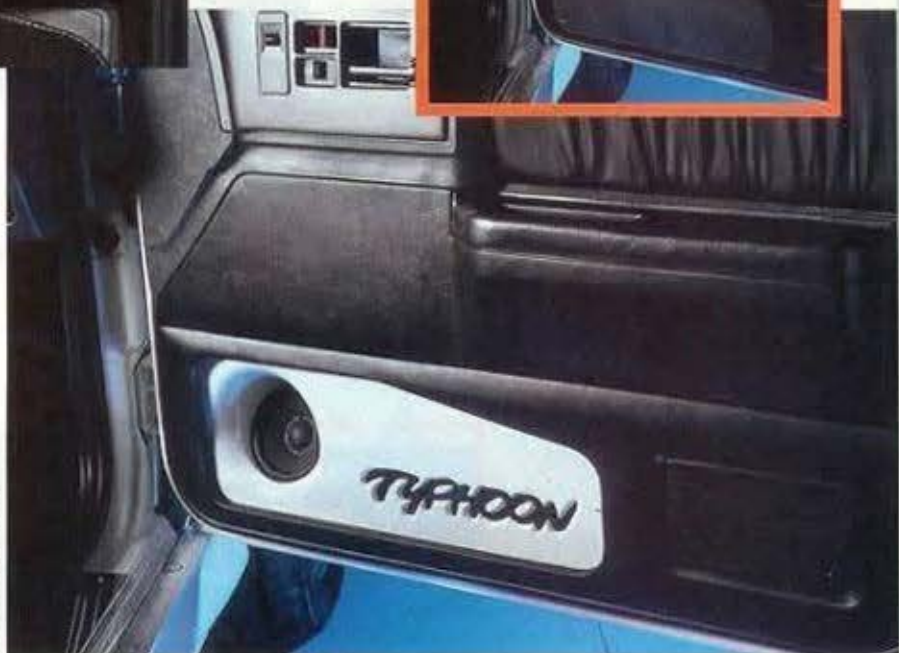
Fiberglass baffle holds 5.25-inch speaker mounted in the bottom of each door.
