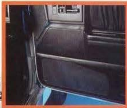
Custom grille made of MDF and metal mesh covers speaker in door.
