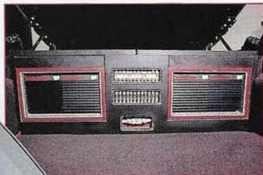
Four of the eight Rockford Fosgate Punch 30's are visible at a glance. A push of a button on the Quantum V.S.E. keypad reveals a whole new set of electronics.
