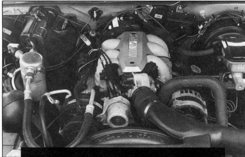
The high performance heart of the Sonoma GT is the L35 195-horse, 4.3L V-6.
