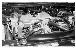
The GMC Syclone comes stock with a 4.3 liter Vortec six-cylinder which is turbocharged and intercooled through an air-to-water heat exchanger. Producing 280 horespower and 350 lb./ft torque from the factory, the Syclone carrying Dave and his daughter CaraMia will run a quick 13.50 in the quarter mile. That's movin'!
