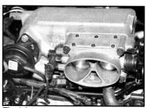
The inlet system incorporates the highflow throttle body from the 5.7L L98 Corvette engine.
