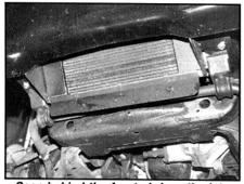
Seen behind the front airdam, the intercooler heat exchanger incorporates a lower lip to help direct air through its core. No doubt an intercooler stone guard will be one of the first aftermarket products out next year.
