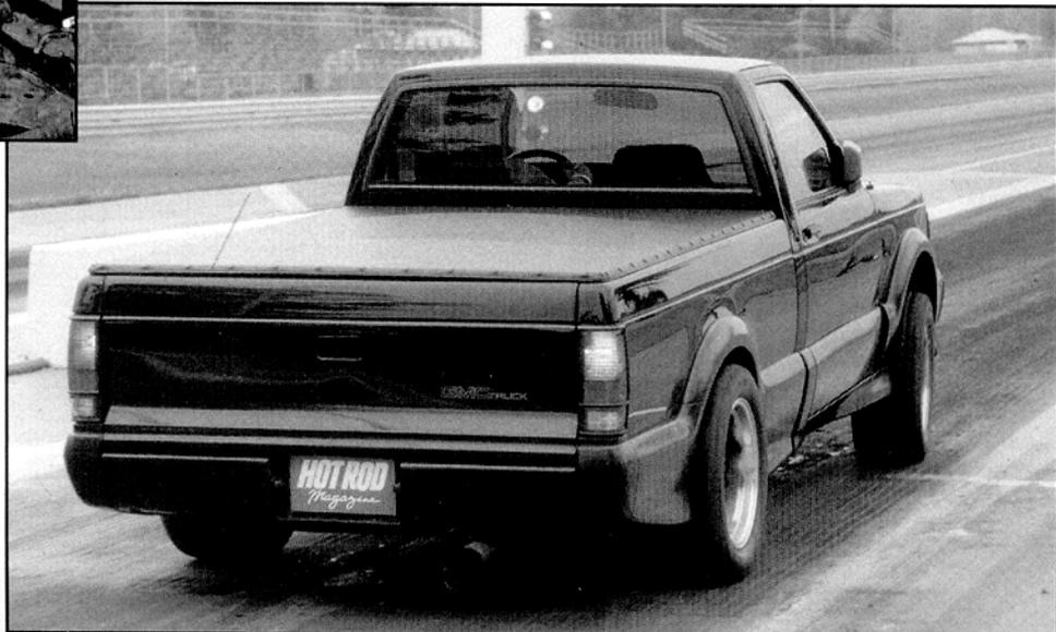
Because the front wheels also provide drive, the Syclone does have some torque steer at launch (see front tire), but it's easily managed.
