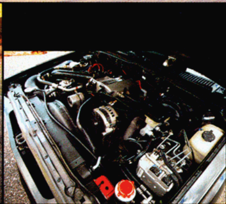
No Bowtie block here. The engine room looks surprisingly stock for a 10-second performer. Of particular note is the 3-inch tubing leading to the throttle body from the KB Big Boy intercooler hidden beneath.
