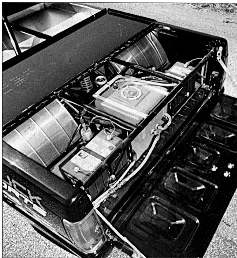
While the sidewalls of the truck's bed remain, the flooring was replaced with modified Alston Engineering aluminum panelling. The rollage rear braces now extend out through the back of the cab and mount above the rear end. A flat panel hinged just in front of the GMC Truck Motorsports lettering gives access to the fuel cell and Delco battery.
