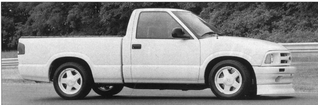
That front spoiler wouldn't last one trip through the Hardee's drive-up lane, but the ride height and stance of the S10 AWD are real-world usable. Based on a 4WD pickup, the front suspension has a wider stance than 2WD versions. A set of 16-inch '92 Camaro wheels were used on this truck, and a modification of the design will be offered on the regular '96 production S10 with the ZQ8 handling package.
