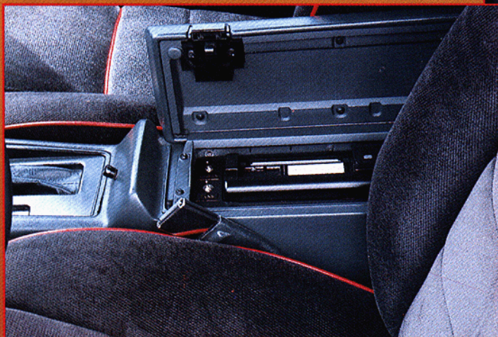
BELOW - Center console holds an Alpine six-disc changer that sends its digital output to the Audio Alchemy jitter reduction machine and then the D/A converter.
