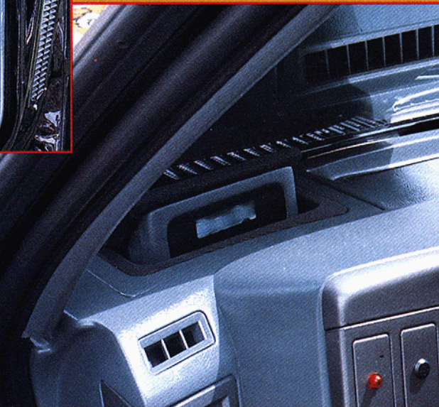
ABOVE - The driver's side speaker location is filled with a motorized Alpine remote display. At the touch of a button, you've got a head-up display. When it's off, the display motors down and there's nothing there.
