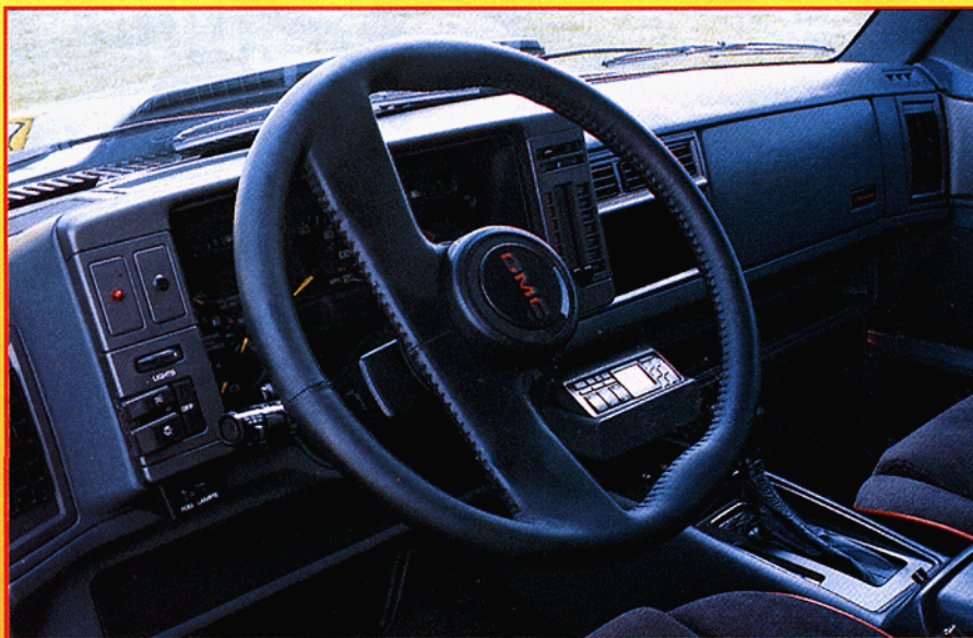
The entire lower section of the dash was removed and replaced with a custom piece that holds an Alpine controller and a pair of USD Waveguides in a position that's much higher and more forward than usual.
