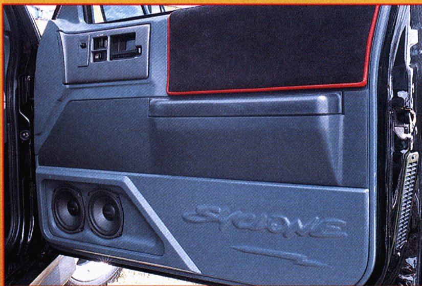
The stock doors were reworked to hold a pair of JL Audio 5.25s each. The Scorpion logo was also worked for looks.
