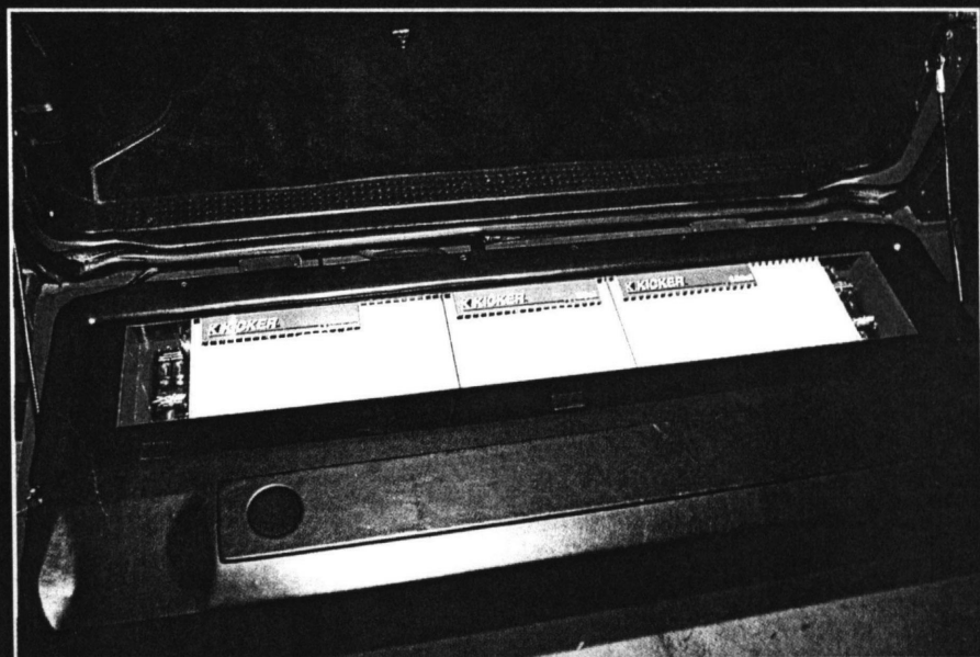
Three of Kicker's new module design amplifiers are mounted in the Typhoon's tailgate. The whole thing is protected with Plexiglas and cooled by a couple of fans.
