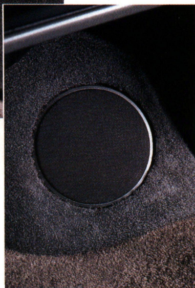
Fiberglass pod added to each kick panel contains MB Quart 6.5-inch midrange (right), protected by panel (above) reinforced with metal grille.
