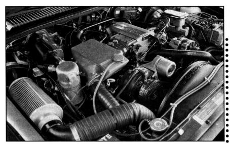
Here's the Kenne Bell-equipped Syclone turbo V6 with all of the performance pieces installed. As you can see, the only visible change is that of the hi-flow air intake and filter (note the low-profile battery used to provide more clearance for the air-intake tube).
