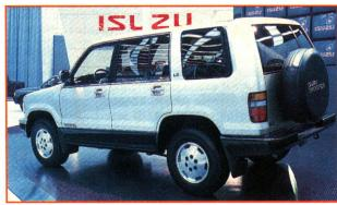
minum 3.2-liter V-6 in both single and double overhead configurations at 175 and 190 horsepower respectively. A four-link/coil spring rear suspension replaces the old Trooper's leaf spring setup while independent double-wishbones are used up front. The Trooper is available with optional all-wheel ABS braking and comes standard with rear-wheel ABS. Isuzu hopes to give the top-of-the-class Ford Explorer a good run for the money with this upscaled Trooper.
