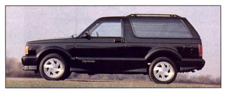
Vehicle type: front-engine, four-wheel-drive, 4-passenger 3-door wagon
