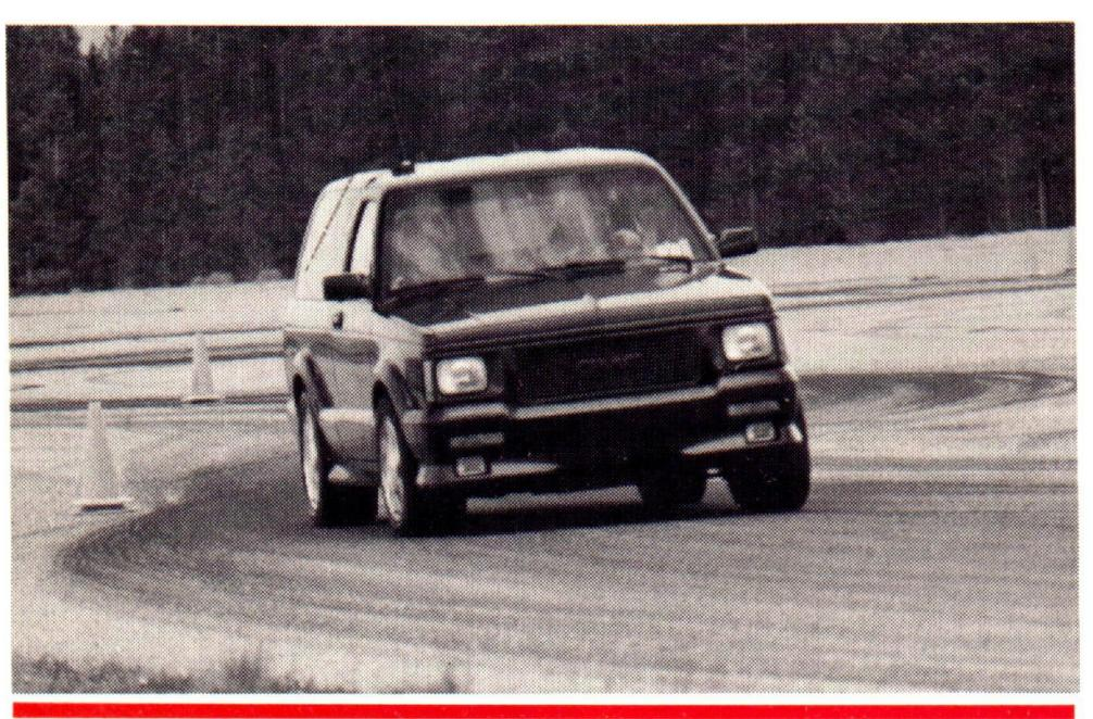
Standard 245/50/16 tires mounted on 16 x 8-inch wheels yielded excellent traction under virtually all driving conditions. Using a tight slalom course at West Yellowstone airport to test the Typhoon's handling, we saw a very forgiving vehicle that both experienced and "not so experienced" drivers felt comfortable with.
