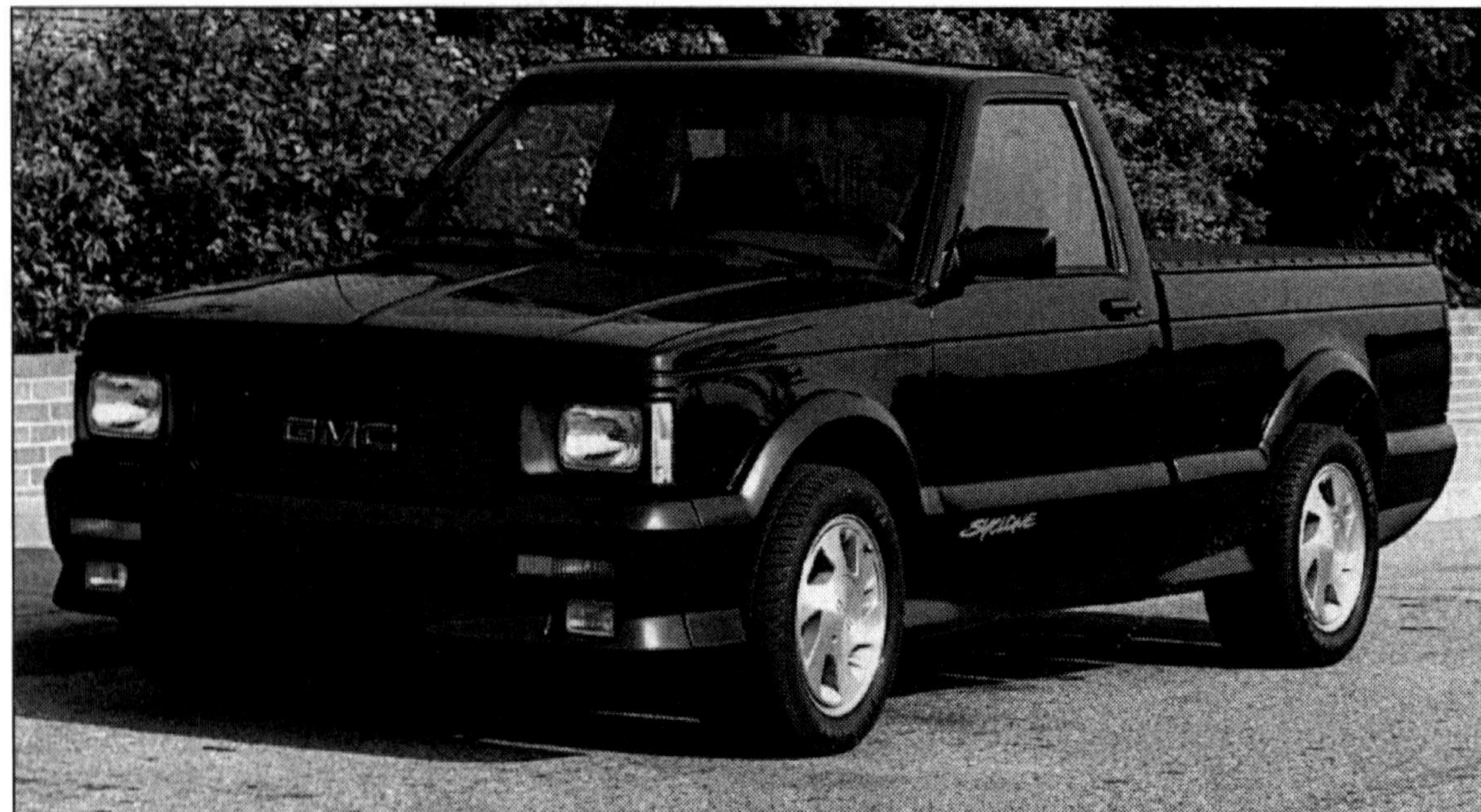
Back for 1992 with minor detail refinements, the GMC Syclone is still one of the fastest production vehicles on the street. All-wheel-drive and a 280-hp turbocharged V-6 engine allow the Syclone to terrorize sports cars that cost twice as much.
