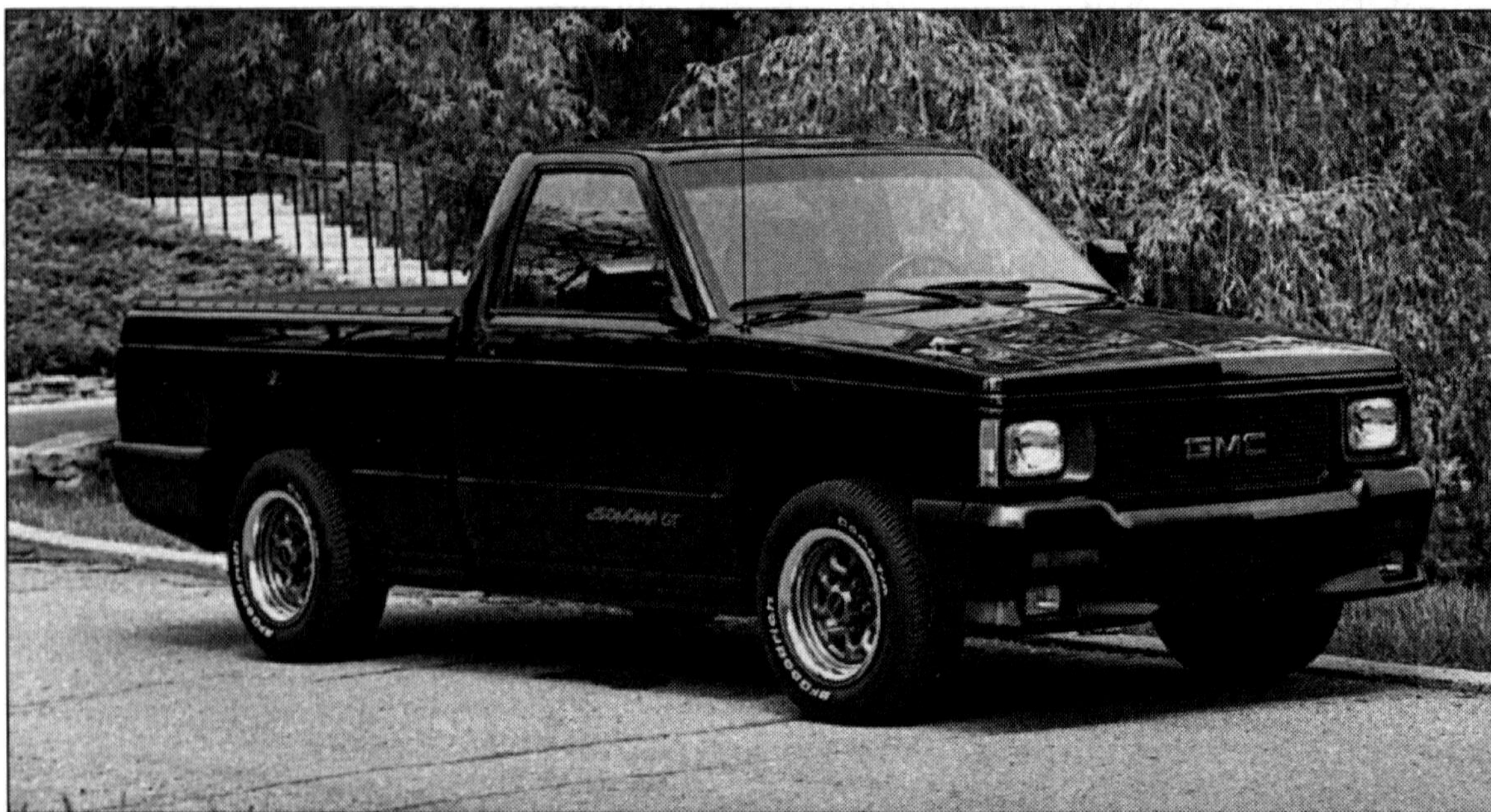
Limited production, high-horsepower output and moderate price are the main features of the new '92 GMC Sonoma GT. The GT is the first truck equipped with GMC's L35 4.3-liter high-performance V-6 engine. Even without a turbocharger, the new engine puts out a whopping 195 horsepower.
