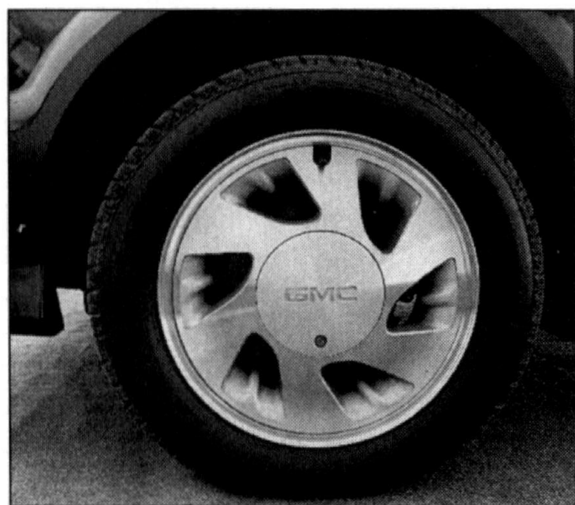
The Typhoon and Syclone roll on Syclone-styled, 16x8 cast aluminum wheels that are wrapped with road-hugging Firestone low-profile radials.
