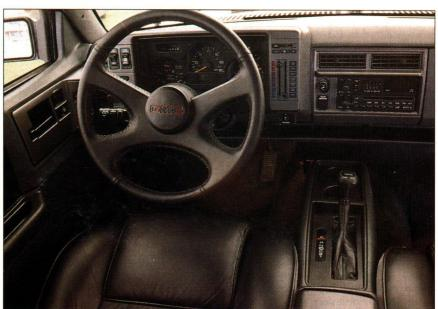
The eye of the Typhoon is thoroughly gussied up with full analog instruments, leather upholstery, sport steering wheel, and power everything. Front buckets have inflatable lumbar supports. In lieu of an airbag, GMC provides three-point seatbelts and a special self-aligning steering-wheel hub. Air conditioning, AM/ FM/cassette stereo, and a graphic equalizer are all standard equipment. A compact disc player is optional.
