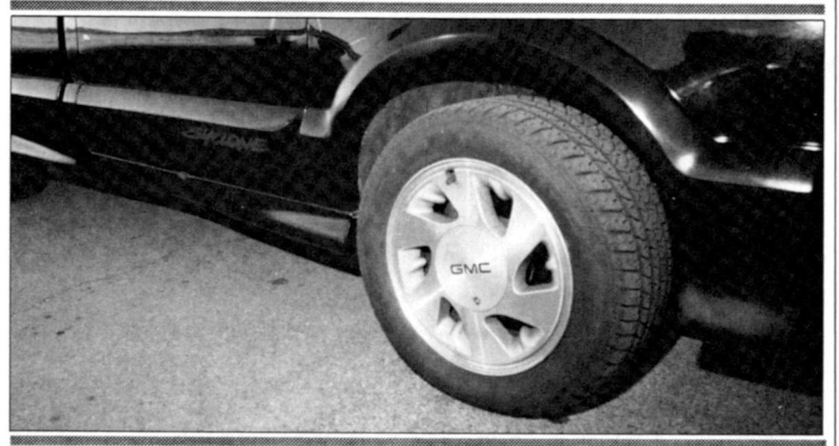
Helping with traction 245/50 VR 16 Firestone rubber all around transmits the power to the ground from the 700R4 transmission coupled to a Borg Warner transfer box. The 3.42 ratio should prove ideal for both cruising and acceleration testing with any reasonable increases in performance.
