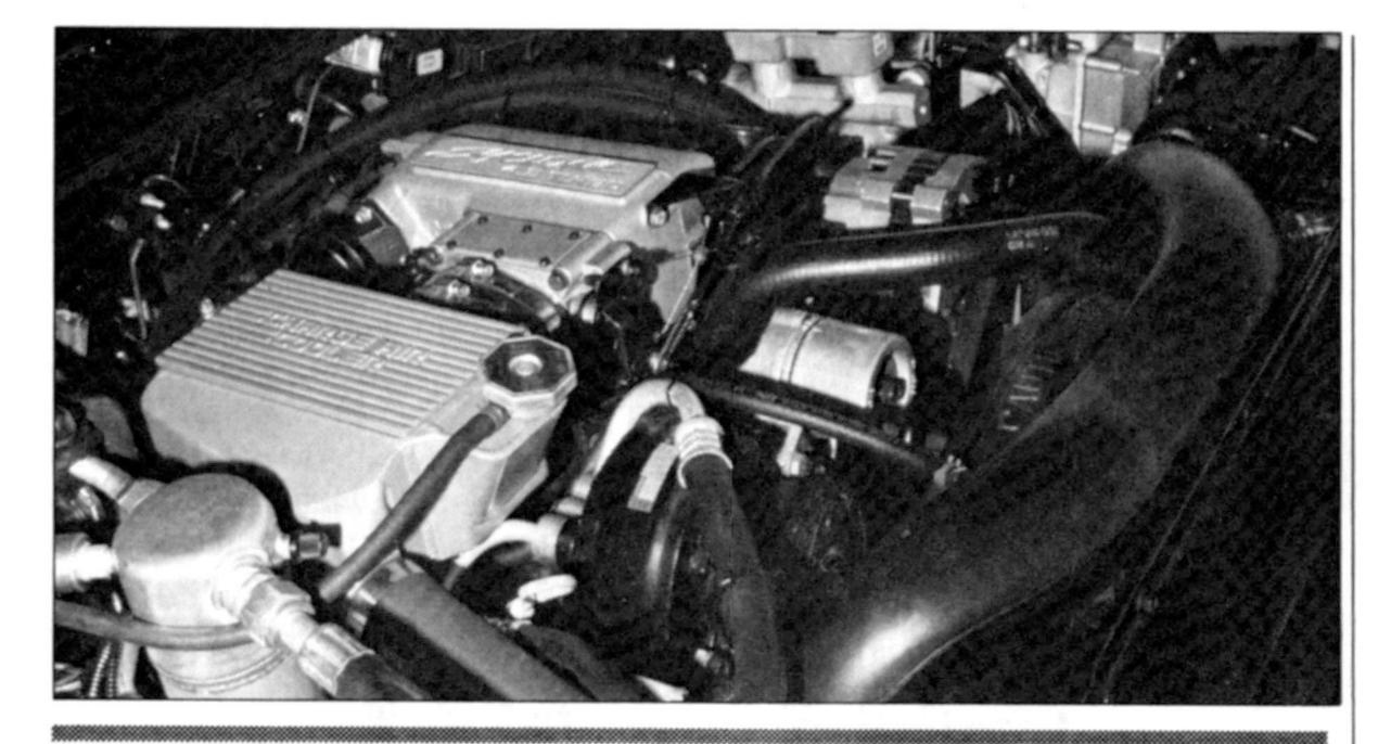
Utilizing direct port injection and a large 350 TPI throttle body the Syclone boasts 280 horsepower in stock form. The sizing of the air/water intercooler below is slightly questionable at this time, but we have valid reports that just about every one of our current Buick performance advertisers have Syclones on order and our guess would be that 10-second Syclones could happen as early as October.
