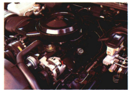
The 7.4-liter V-8 in the 454 SS (near right) is massive and mean. The Syclone's turbocharged V-6 (far right) is smaller but more powerful.
