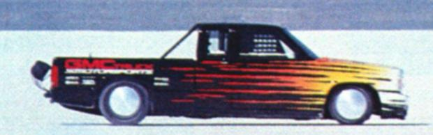
with a new and improved truck, the Syclone LSR (for land-speed record). The basic layout of the LSR is similar to the older ETV: Both trucks ran with modified 4.3-liter, 90-degree V-6 engines driving the rear wheels. The engines were bored and stroked to displace 5.0
