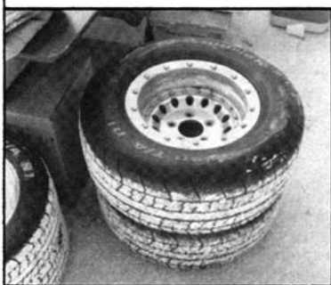
ABOVE LEFT — BFGoodrich tires were shaved down for the salt track. Unlike many special applications used on the salt, these Comp T/A R1 radials are DOT approved street legal. The tires are "Z" speed rated.
