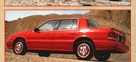
Aimed directly at Ford's SHO Taurus, the Spirit is a four-door, high-performance sedan, with emphasis on performance. With a 220-horse, DOHC turbo-charged and intercooled 2.2- liter four cylinder, the R/T scoots from 0-60 in 6.8 seconds—fast enough to devastate the Hi-Po Taurus. And, because of its twin balance shafts, the engine sings easily to red-line—which is 6500rpm—although Chrysler engineers claim the low-friction valvetrain is capable of 8000rpm!
