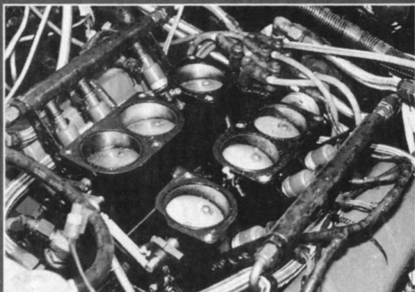
Not your normal fuel injection, a special set of six-throated Kinsler fuel injection throttle assemblies and manifold went on the 5.0-liter V6.
