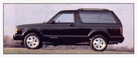
Vehicle type: front-engine, four-wheel-drive, 4-passenger, 3-door wagon
